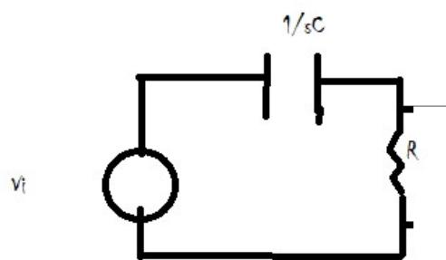
$$\begin{aligned} V_i(s) &= V_R(s) + V_c(s) = R * i(s) + \frac{1}{sC} i(s) = i(s) \left( R + \frac{1}{sC} \right) = V_c(s) * sC \left( R + \frac{1}{sC} \right) = V_c sC \left( \frac{sRC + 1}{sC} \right) \\ &= V_c (1 + sRC) \end{aligned}$$
