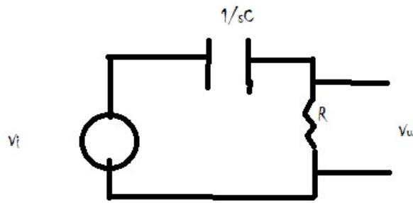
$$V_i(s) = i(s) \left( R + \frac{1}{sC} \right) = \frac{V_R(s)}{R} \left( R + \frac{1}{sC} \right) \quad G(s) = \frac{V_R}{V_i} = \frac{sRC}{(sRC+1)}$$
